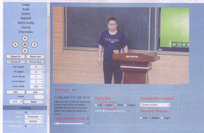
**Close:** The close-up image includes tracking the target above the waist, as shown in the following figure.
