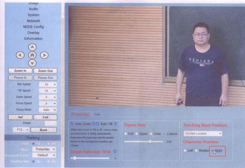
**Step 5** According to the requirements of the application scenario, you can choose whether to require “Humanoid frame” and “Tracking hint”, with default modes.
