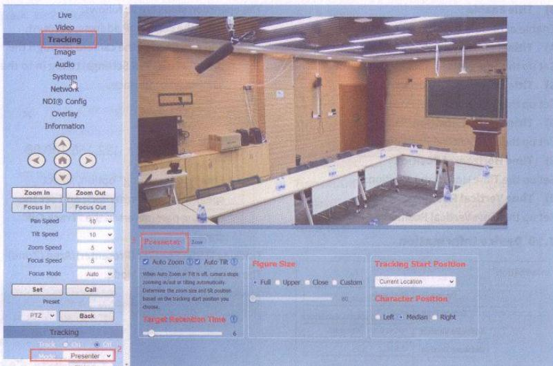
**Step 3** We can consider how long the Target Retention Time will take, with a default of 6 seconds and a maximum of 10 seconds.
