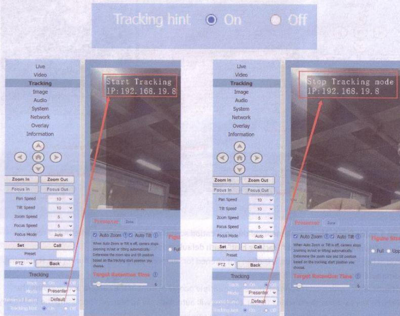
**Step 6** Turn on tracking, press the arrow keys to select the tracking target, and then press Home to confirm.
