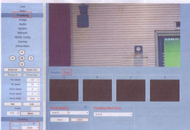
**Step 3** Use the web interface's directional keys and Zoom In/Out to adjust the lens position, and set multiple preset positions such as Zone A successively, and click "Save".
