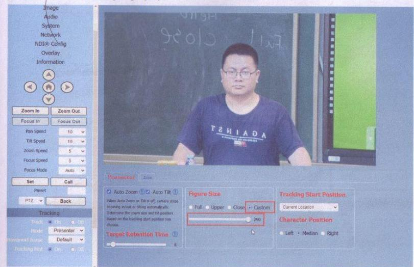
**Note:** When Auto Zoom or Tilt is off, camera stops zooming or tilting automatically. Determine the zoom size and tilt position based on the tracking start position you choose.
